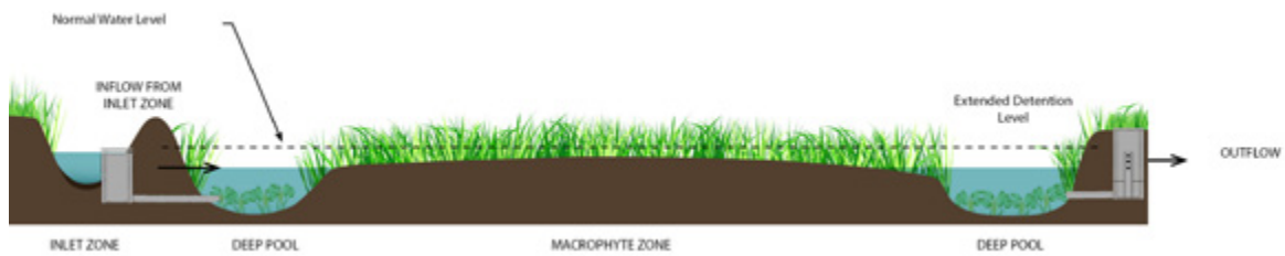
Figure 16: Typical wetland longitudinal section
