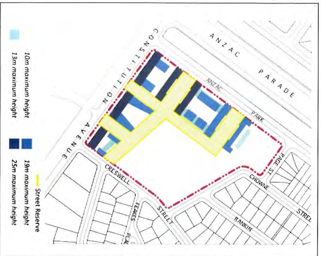
Figure 2 Diagram showing building height restrictions for the Campbell Section 5 development, Constitution Avenue which must be adhered to (pursuant to condition 4 a) of this decision notice).
