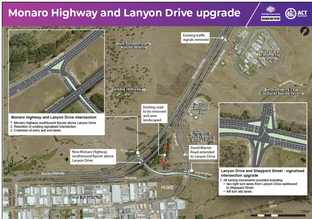
Figure 6 Monaro Highway and Lanyon Drive upgrades
