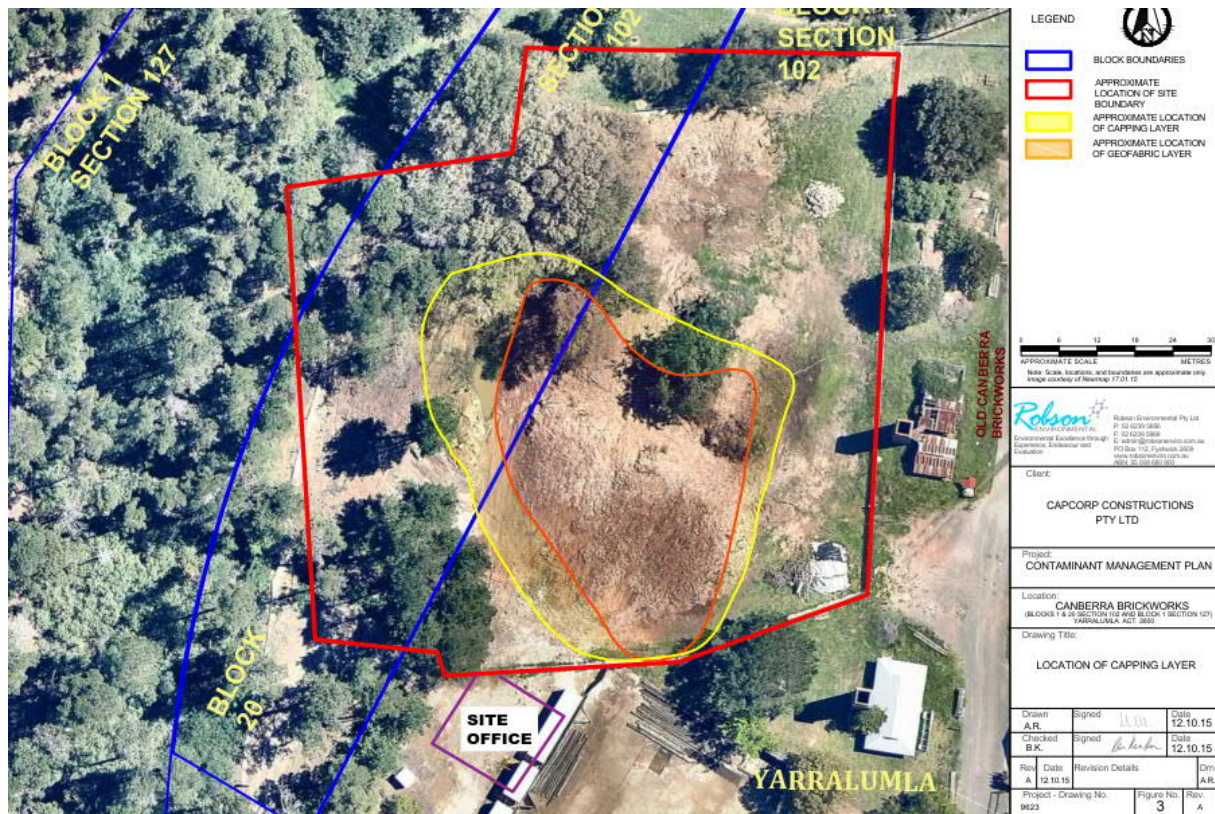
Figure 6 Location of Asbestos Dump capped area (extracted from Robson, 2015)
