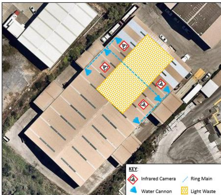
Figure 3: Light Waste Fire Suppression Schematic
