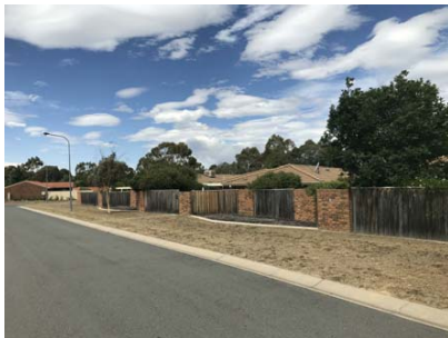
3. BLOCK 14 SECTION 19, RZ1 SUBURBAN ZONE, MIX OF 9 SINGLE LEVEL DETACHED RESIDENCES. WALL AND COURTYARD FENCE ARRANGEMENT ARE BUILT WITH ZERO SETBACK TO THE BOUNDARY. SETBACK GARDEN BEDS PROVIDE SOME ARTICULATION TO THE STREET FRONTAGE.
