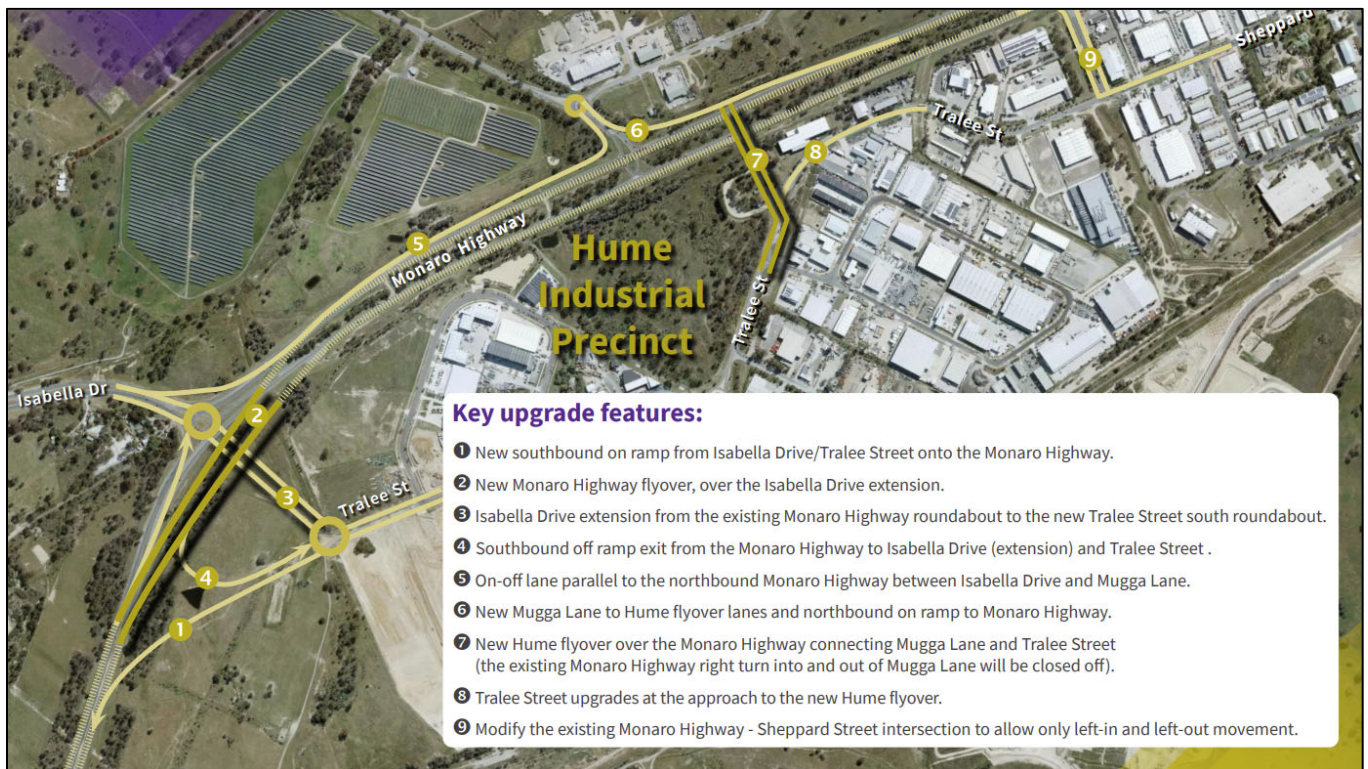
Figure 4.1 Proposed Monaro Highway intersection upgrade
