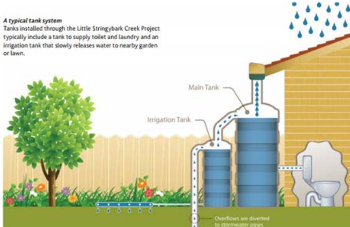
Figure 9 Example of a typical tank system
