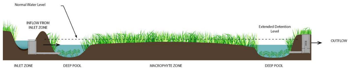
Figure 16 Typical wetland longitudinal section
