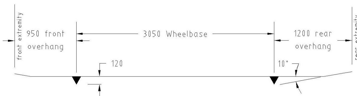
Figure 5.1 – B99 vehicle template for new driveway design (NTS) Domestic and Commercial
