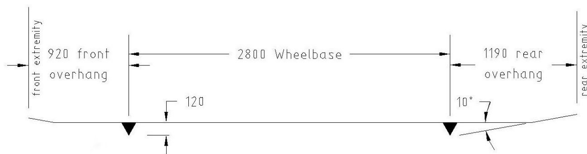
Figure 5.2 – B85 vehicle template for driveway construction (NTS) Domestic Driveways only (Subject to Roads ACT approval)
